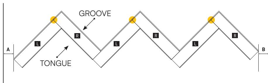
Finish the first row up to the wall. Allow for an expansion gap of 10 mm along each wall on both sides.
