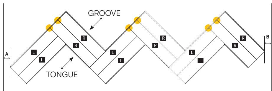
Finish the first row up to the wall. Allow for an expansion gap of 10 mm along each wall on both sides.
