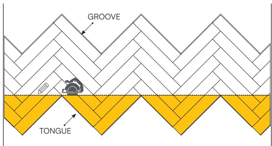
Push the sawn-off floor towards the wall, leaving a 10 mm gap.
