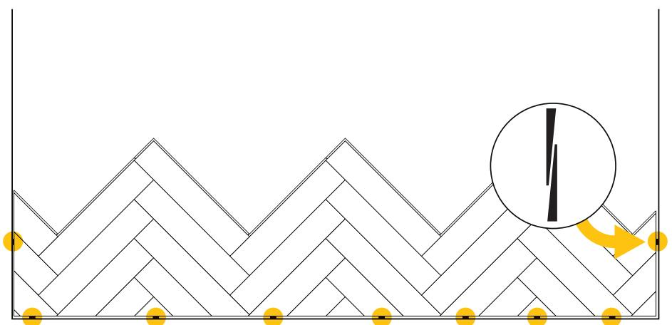
Use the saved sawn-off pieces to complete the installation on the other side of the room.
