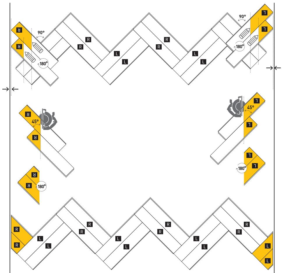
Rotate the right-hand plank 180°, then mark it and saw it at a 45° angle. Rotate the sawn-off pieces 180° and click them into the first planks.
