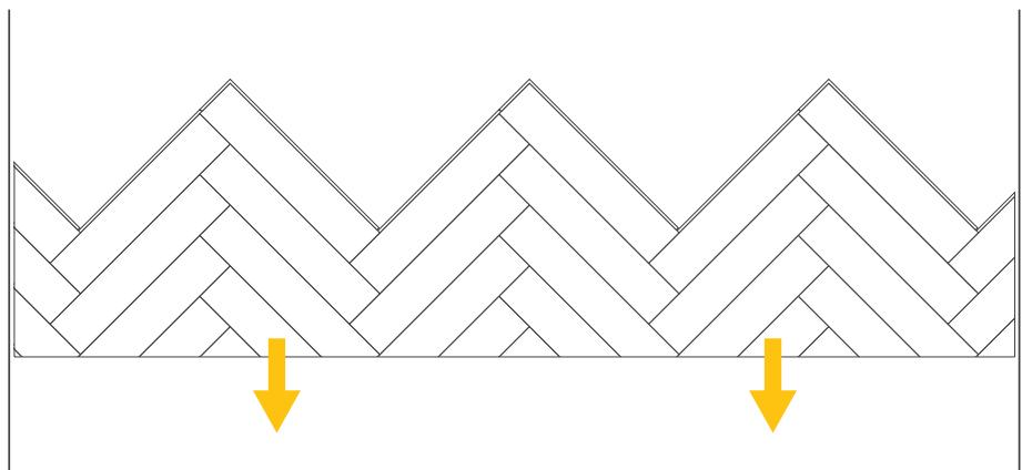
Place spacer blocks between the wall and the floor. Continue finishing the floor.
