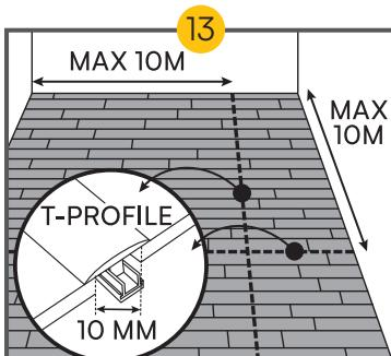
Parky is a real wood floor. Sufficient expansion gaps should therefore be left along each wall, around heating pipes, and around obstacles on the surface (door frames, for example).
